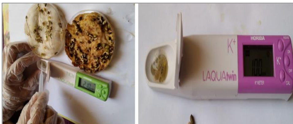
Fig 6b: Potassium and Nitrate determination by HORIBA NO3 and K Meters
